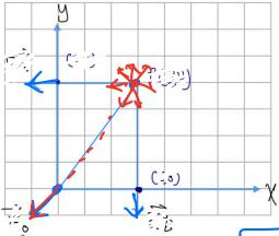
Q2) Consider the field  $\vec{E} = -\frac{xy^2}{18} \vec{a}_y$ . Sketch the field components at P(x=4, y=3, z=5) in x-y and  $\rho$ -z planes. From the graph measure the following components:
