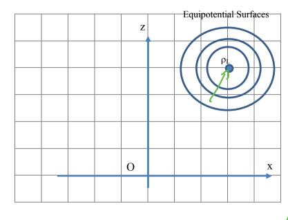
Equipotential surfaces are cylinders with axis at x=3 and z=4
